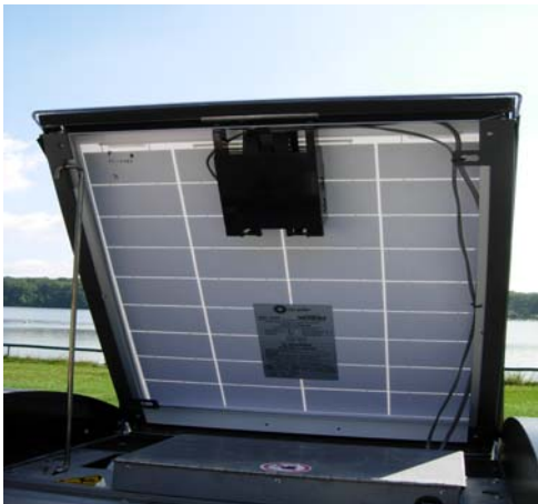
The lid is a solar panel. The solar covering is made from a polymer than can take the force of a baseball bat, in case vandalism is an issue.
